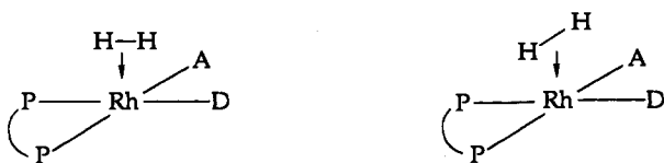
Figure 2. Possible modes of H 2 addition to cis -diphosphino Rh(I) complexes containing donor/acceptor ligands. Left, disfavored approach; right, favored approach.
